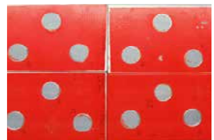
ZINGA + Zingaceram HS + Zingaceram PU after 720 h condensation (above) and 1440 h salt spray (under)
