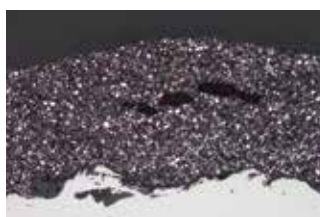
Copper particles blend in two layers of ZINGA
