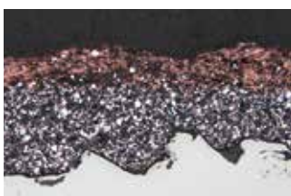
Copper particles on top of ZINGA
