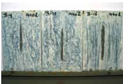
ZINGA 2 x 90 µm DFT after 720 h condensation (above) and 1440 h salt spray (under)
