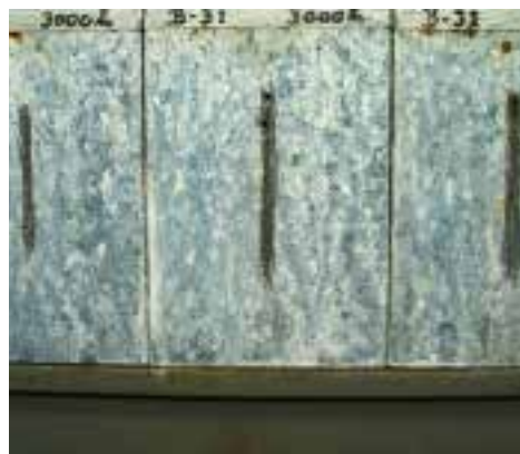
ZINGA 2 x 90 µm DFT after 3000 h salt spray
